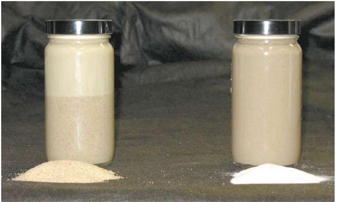
Figure 1. Suspension problems with coarse sand.
